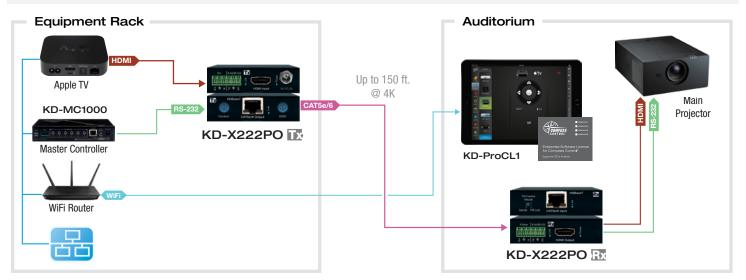
\* For all installations, we highly recommend use of KD-CAT6STP1X STP cabling, especially in hostile electrical environments. The shield of CAT6STP must be soldered on both ends to the shield of RJ45 connector used. The CAT5/5e/6 cable has to be terminated according to TIA/EIA-568-B standard. The use of STP CAT5, 5e is not recommended.
